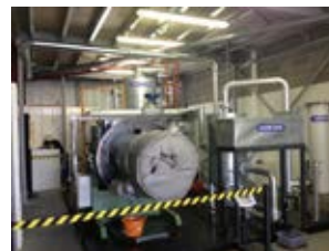
The operational pilot scale facility for processing 50kg batches of waste
